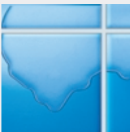
The water spreads as a thin film on the surface and lifts dirt from the surface ...
